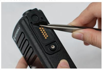
Figure 5-20. UC escutcheon removal
