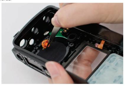
Figure 5-24. Emergency button removal
