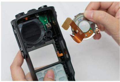
Figure 5-22. Speaker assembly removal
