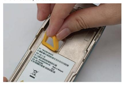
Figure 5-12. Battery contact seal removal
