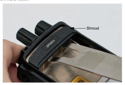
Figure 5-3. Shroud removal
