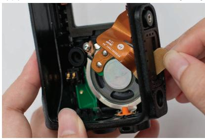
Figure 5-21. UC flex removal
