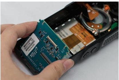
Figure 5-18. Keypad board removal
