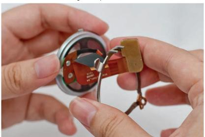
Figure 5-28. Speaker retainer reassembly
