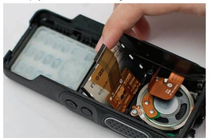
Figure 5-31. Display module reassembly
