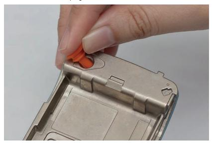
Figure 5-13. RF rubber plug removal
