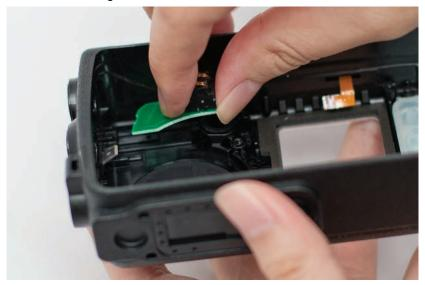
Figure 5-25. Bluetooth GPS antenna removal
