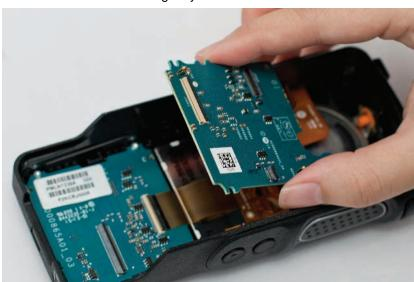
Figure 5-17. Interface board removal
