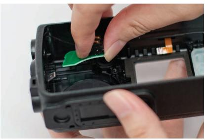
Figure 5-26. Bluetooth GPS antenna reassembly
