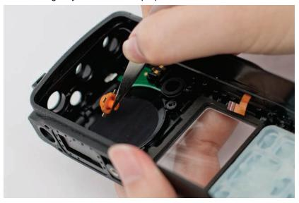
Figure 5-27. Emergency button reassembly
