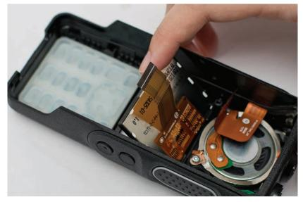
Figure 5-19. Display module removal
