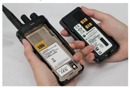
Figure 5-1. Battery removal
