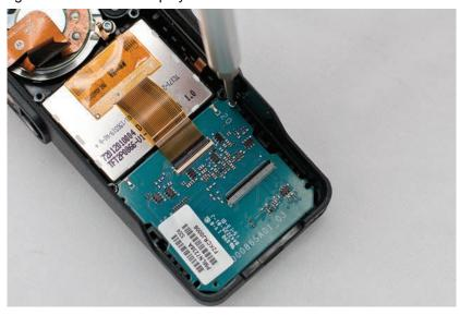
Figure 5-32. Keypad Board reassembly
